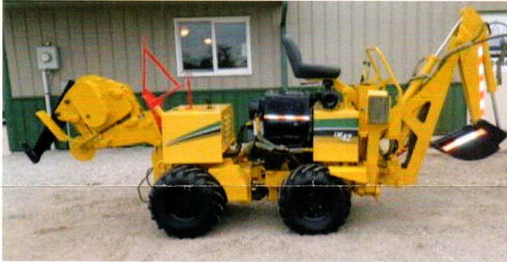
Picture #1: Service drop plow
